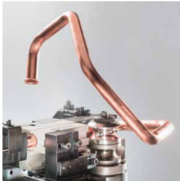
5. There are multiple types of bending available. Compression bending (extremely fast), to make 'elbows' and 'S' and bends near end forms. Draw bending - left or right or variable radius ends. And now including mandrel bending
